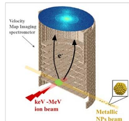
Figure 2: VMI spectrometer
